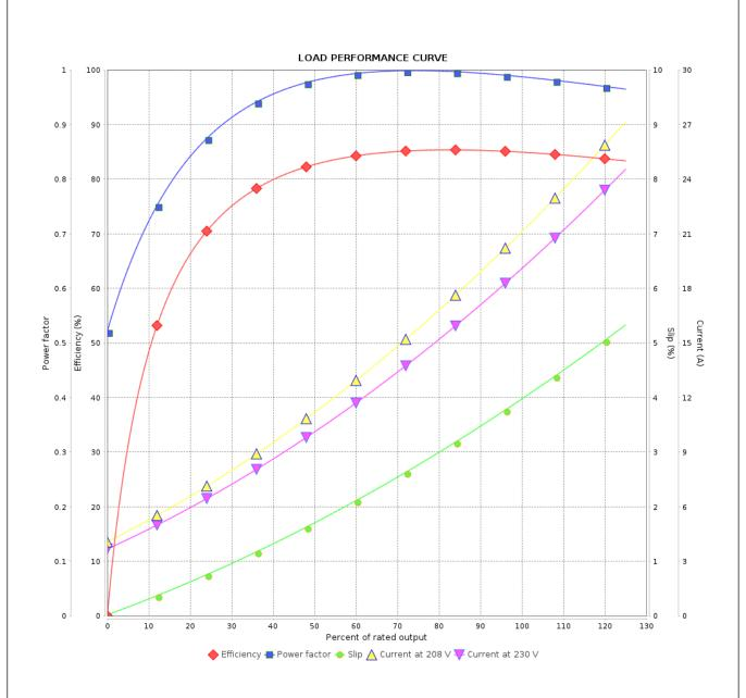
Performance : 208-230 V 60 Hz 2P : 0.0030 kgm<sup>2</sup> Rated current : 21.0-19.1 A Moment of inertia (J) **LRC** Duty cycle : Cont.(S1) : 6.5 Insulation class Rated torque : 1.05 kgfm : F Locked rotor torque : 220 % Service factor
