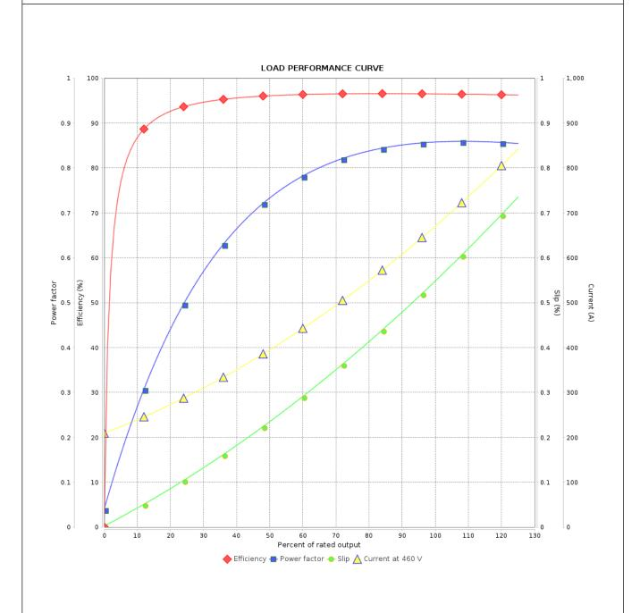
Performance : 460 V 60 Hz 4P Rated current : 665 A Moment of inertia (J) : 9.92 kgm<sup>2</sup> **LRC** : 7.1 Duty cycle : Cont.(S1) Rated torque : 243 kgfm Insulation class : F Locked rotor torque : 229 % Service factor : 1.15 Breakdown torque : 250 % Temperature rise : 80 K Rated speed : 1790 rpm
