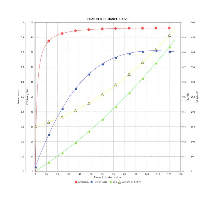
Performance : 575 V 60 Hz 6P : 386 A Rated current Moment of inertia (J) : 15.5 kgm<sup>2</sup> **LRC** : 6.0 Duty cycle : Cont.(S1) Rated torque : 244 kgfm Insulation class : F Locked rotor torque : 200 % Service factor : 1.15 Breakdown torque : 210 % Temperature rise : 80 K Rated speed : 1192 rpm
